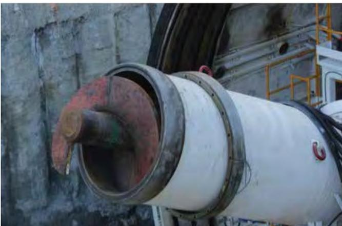
*A screw conveyor moves the material back to the TBM's trailing gear.*
