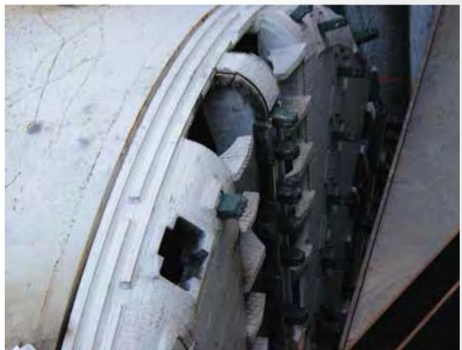
*Any material dislodged by cutter teeth flows through the cutterhead into a chamber behind the cutterhead.*
