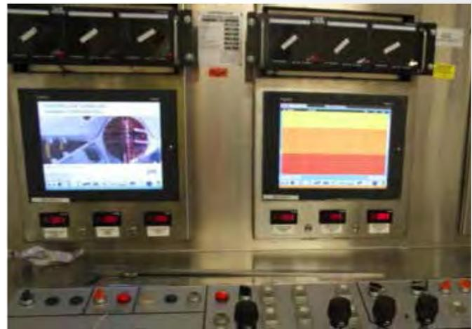
*In the TBM control centre, the TBM operator can monitor key information like pressure on the cutterhead and TBM progress.*
